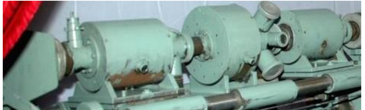
Asia's first Horizontal Transmission Electron Microscope (1946-1948) At display in Saha Institute of Nuclear Physics (SINP)
